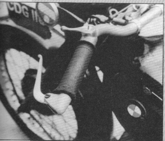
Handlebar controls are of a piece with the result of the design – inverted levers, integrated choke and one-unit horn/dip/twistgrip demonstrate attention to detail.
