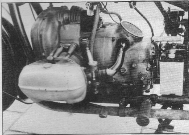
Note the full air filtering and the alloy valve cover (with oil filler cap) – signs that BMW were very conscious of long life and reliability.
